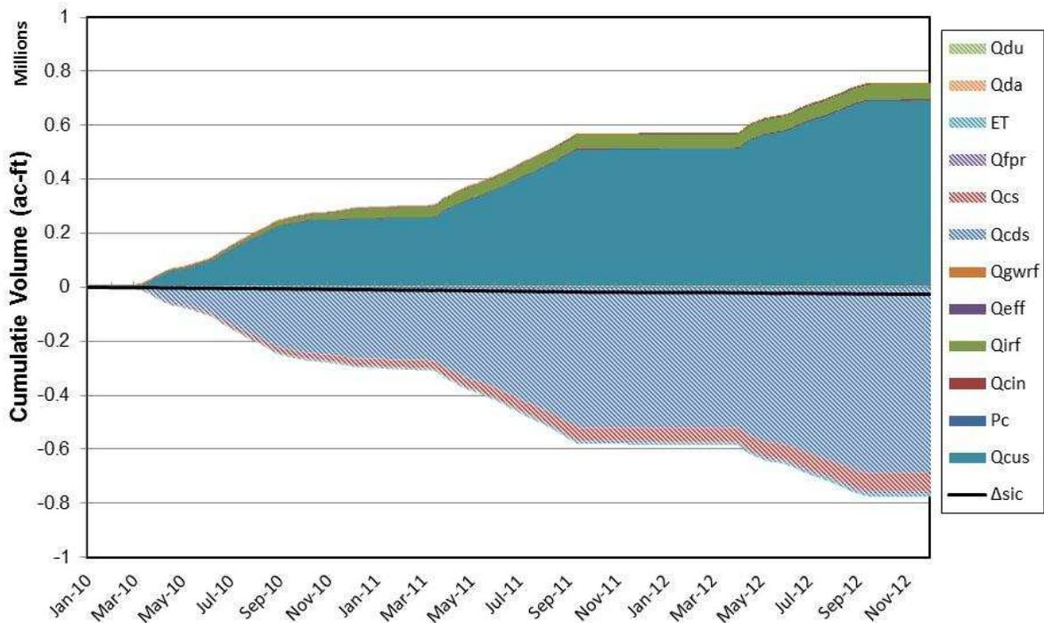
Figure 19. Stacked bar chart showing cumulative volumes of the RGCP-scale channel water budget analysis and the resulting cumulative change in-channel storage in Segment 3
