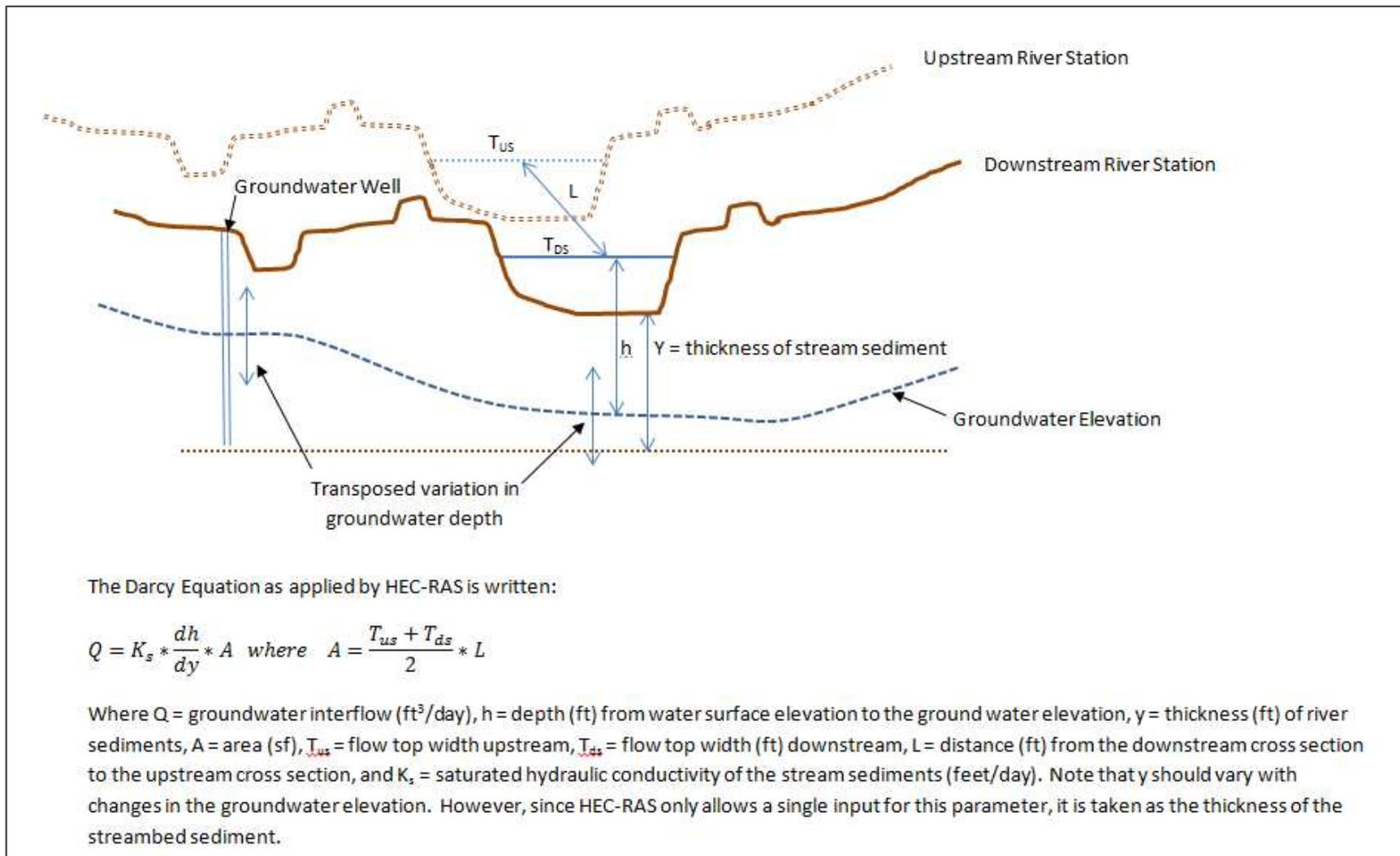
Figure 5. HEC-RAS Groundwater Interflow Schematic
