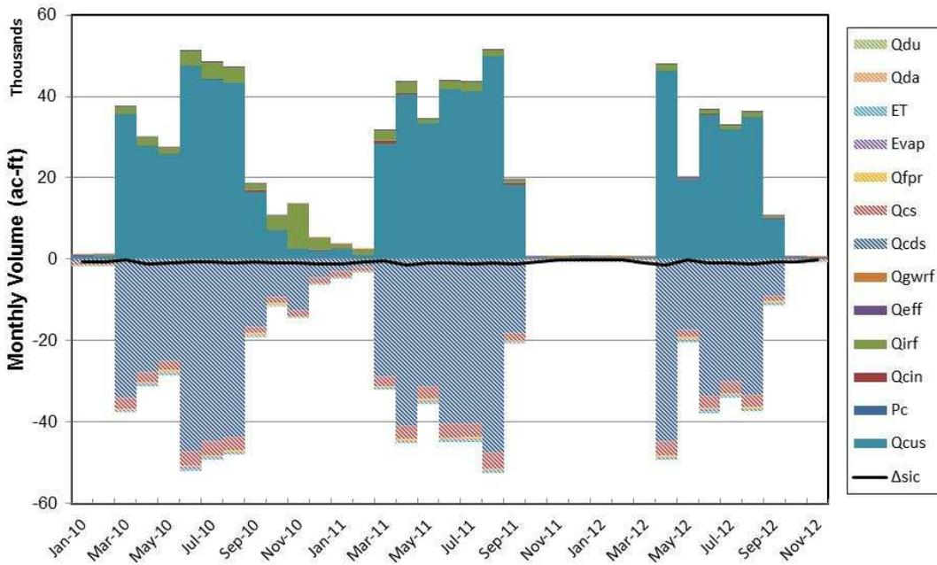
Figure 18. Stacked bar chart showing monthly volumes of the RGCP-scale channel water budget analysis and the resulting monthly change in-channel storage in Segment 3
