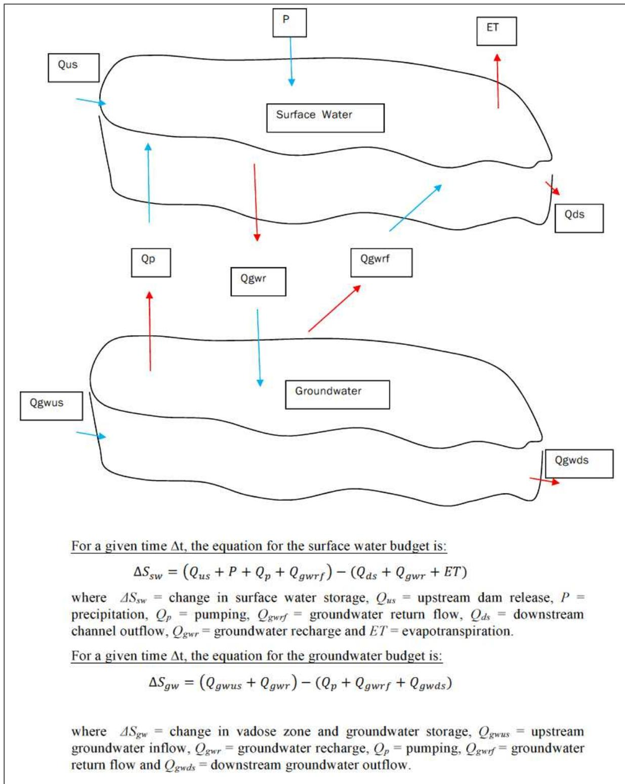
**Figure 13. Local-basin-scale Water Budget Equation and Schematic Diagram (as provided in the Scope of Work) (USIBWC, 2012a)**
