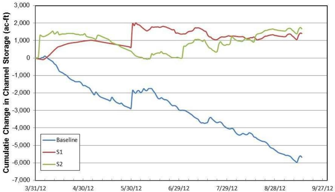
**Figure 26. Cumulative change in-channel storage during 2012 under baseline (actual) conditions and under the hypothetical release scenarios (Scenarios S1 and S2) – Segment 3**
