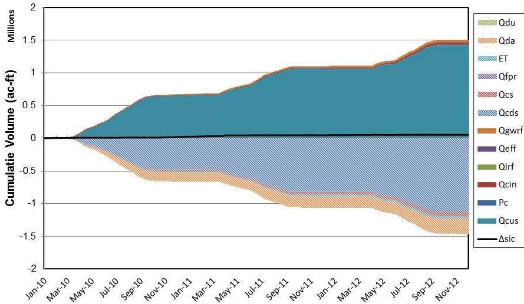
**Figure 15.** Stacked bar chart showing cumulative volumes of the RGCP-scale channel water budget analysis and the resulting cumulative change in-channel storage in Segment 1
