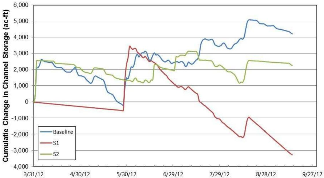
**Figure 24. Cumulative change in-channel storage during 2012 under baseline (actual) conditions and under the hypothetical release scenarios (Scenarios S1 and S2) – Segment 1**
