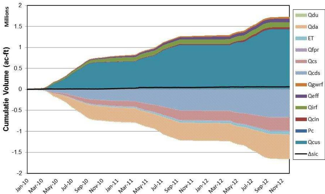
**Figure 23.** Stacked bar chart showing cumulative volumes of the RGCP-scale channel water budget analysis and the resulting cumulative change in-channel storage in the overall RGCP
