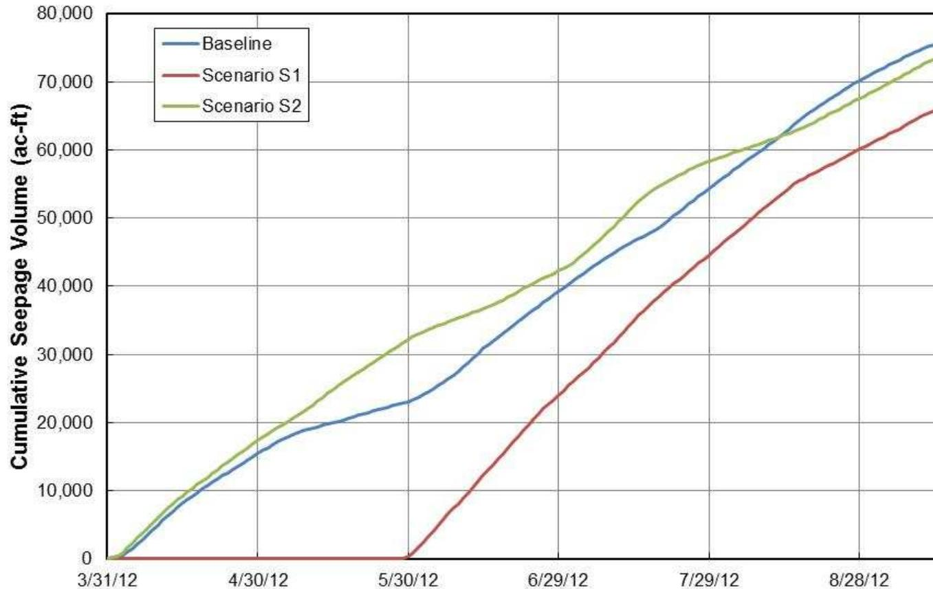
**Figure 8.** Cumulative seepage volumes predicted by the HEC-RAS models for baseline 2012 conditions, and under the Scenario S1 (delayed single pulse) and Scenario S2 (normal single pulse) releases
