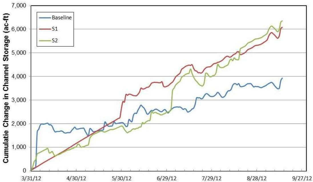
**Figure 27. Cumulative change in-channel storage during 2012 under baseline (actual) conditions and under the hypothetical release scenarios (Scenarios S1 and S2) – Segment 4**
