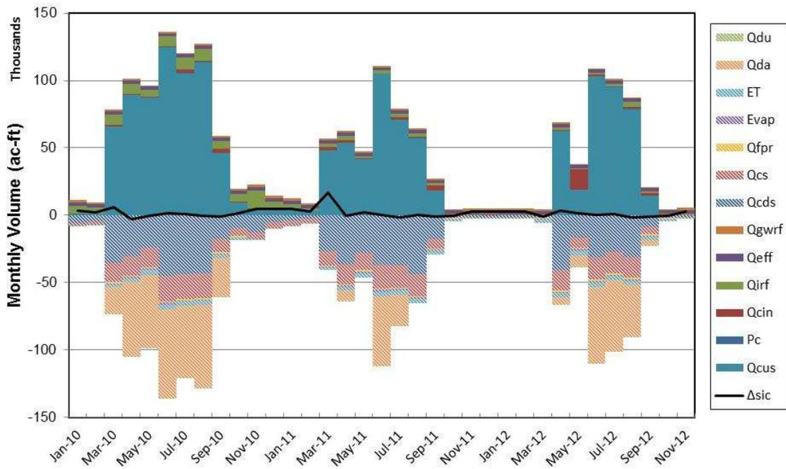
**Figure 22.** Stacked bar chart showing monthly volumes of the RGCP-scale channel water budget analysis and the resulting monthly change in-channel storage in the overall RGCP
