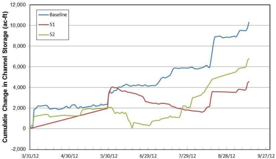
**Figure 25. Cumulative change in-channel storage during 2012 under baseline (actual) conditions and under the hypothetical release scenarios (Scenarios S1 and S2) – Segment 2**
