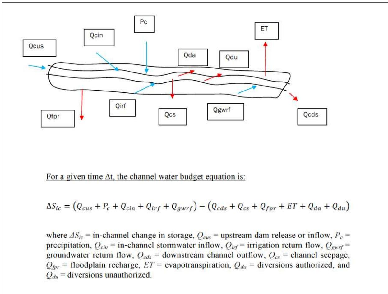
**Figure 9. RGCP-scale Channel Water Budget Equation and Schematic Diagram (as provided in the Scope of Work) (USIBWC, 2012a)**
