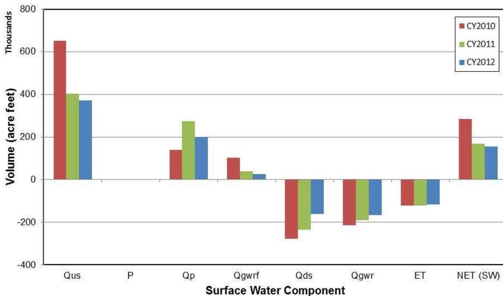
**Figure 29.** Annual and total volume for each component of the local-basin-scale surface-water budget
