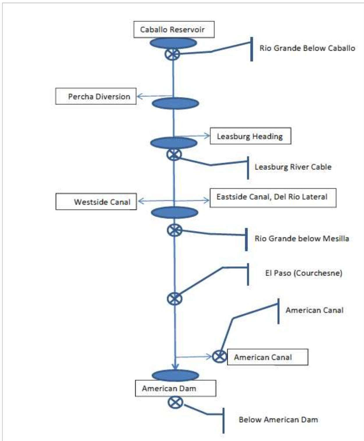
Figure 2. HEC-RAS Model Coverage and Key Locations
