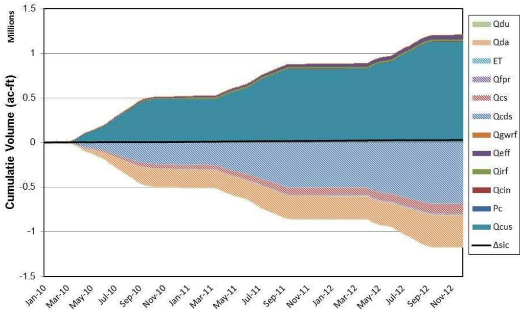
Figure 17. Stacked bar chart showing cumulative volumes of the RGCP-scale channel water budget analysis and the resulting cumulative change in-channel storage in Segment 2
