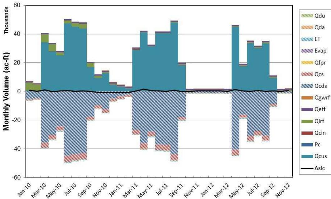
**Figure 20. Stacked bar chart showing monthly volumes of the RGCP-scale channel water budget analysis and the resulting monthly change in-channel storage in Segment 4**
