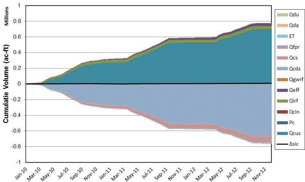
**Figure 21. Stacked bar chart showing cumulative volumes of the RGCP-scale channel water budget analysis and the resulting cumulative change in-channel storage in Segment 4**
