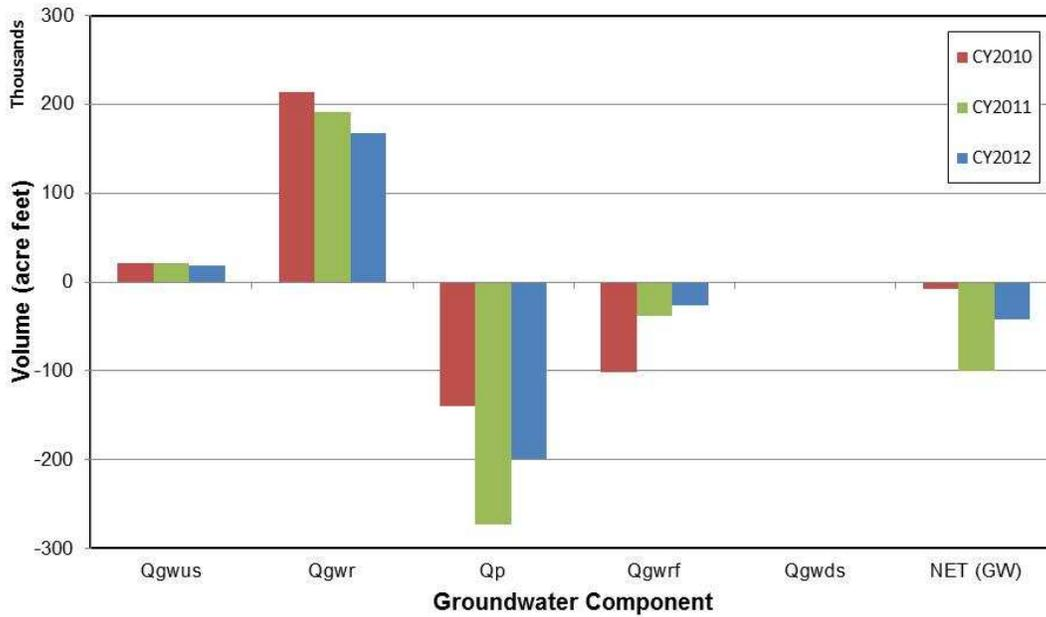
**Figure 30. Annual and total volume for each component of the local-basin-scale groundwater budget**
