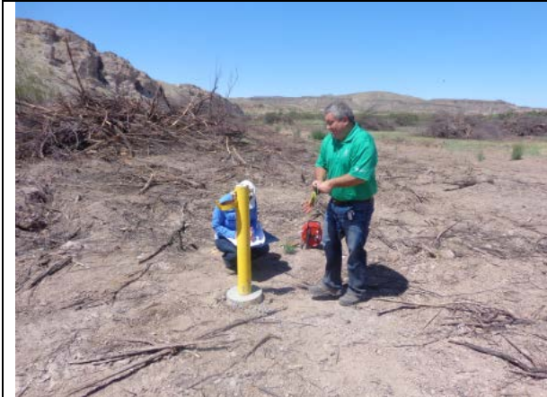
Monitoring groundwater levels at the new Selden Point Bar wells with contractor, May 21, 2014
