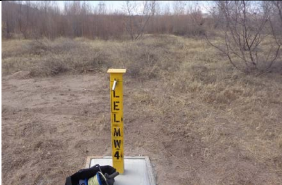
New well 4 drilled outside of the tree planting area to avoid damage to the well. Feb 2019
