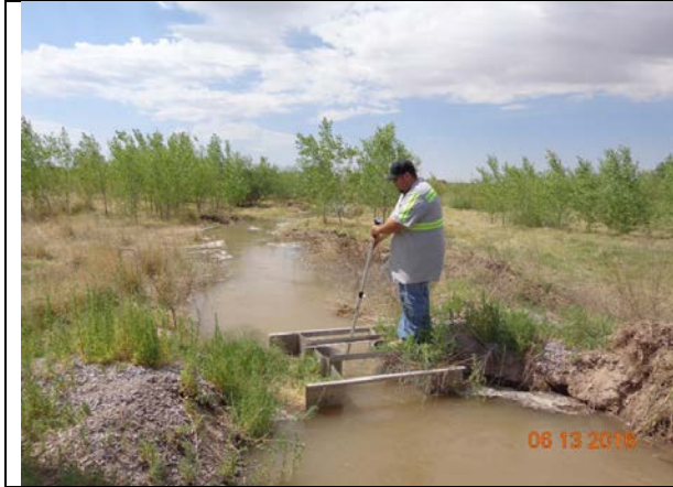
EBID hydrologist collects flow data to estimate water deliveries, June 2016
