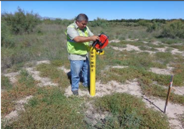
Contractor from HDR conducts groundwater monitoring, September 2013
