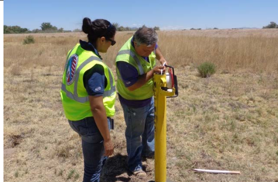
Contractors train USIBWC on groundwater monitoring and sonde data retrieval at the same site, June 2013
