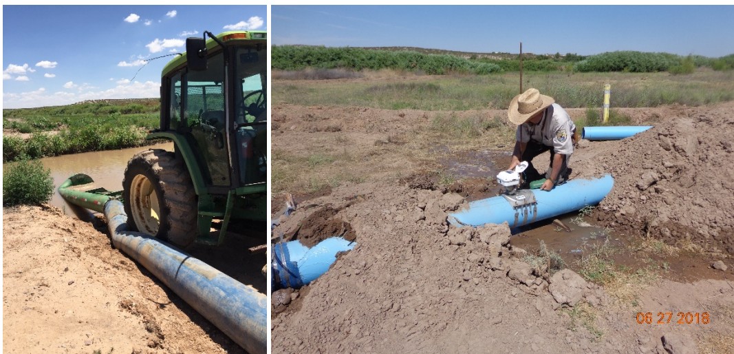
Figure 25 USIBWC's gator pump and tractor enabled Mesilla East site to be irrigated from the California Lateral (left); USFWS reads the meter during the June 2018 irrigation (right).
