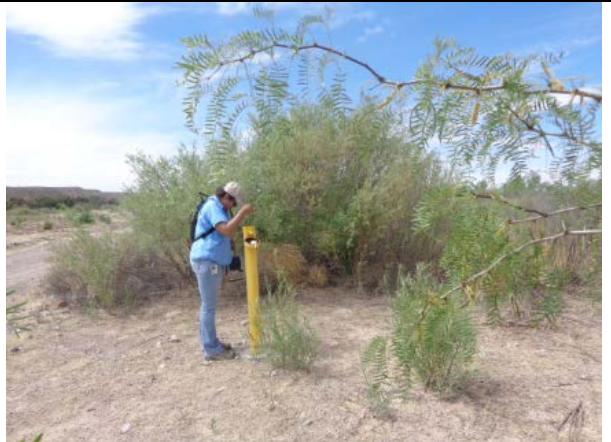
USIBWC conducting groundwater level monitoring prior to irrigation releases, May 2014
