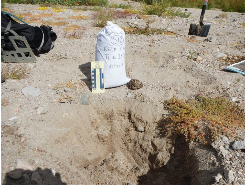
Photo A.53. View of bed material along the channel bed of Horse Canyon Creek that was collected in Sample S12.
