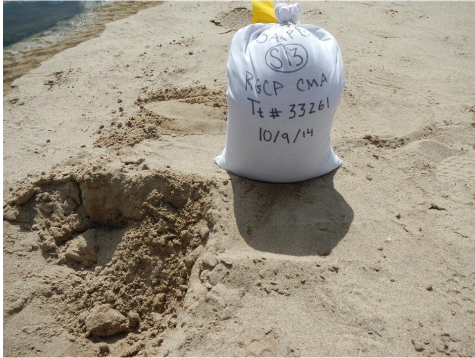
Photo A.83. View of the bed material along the alternate bar upstream from the Anapra Bridge that was collected in Sample S13.
