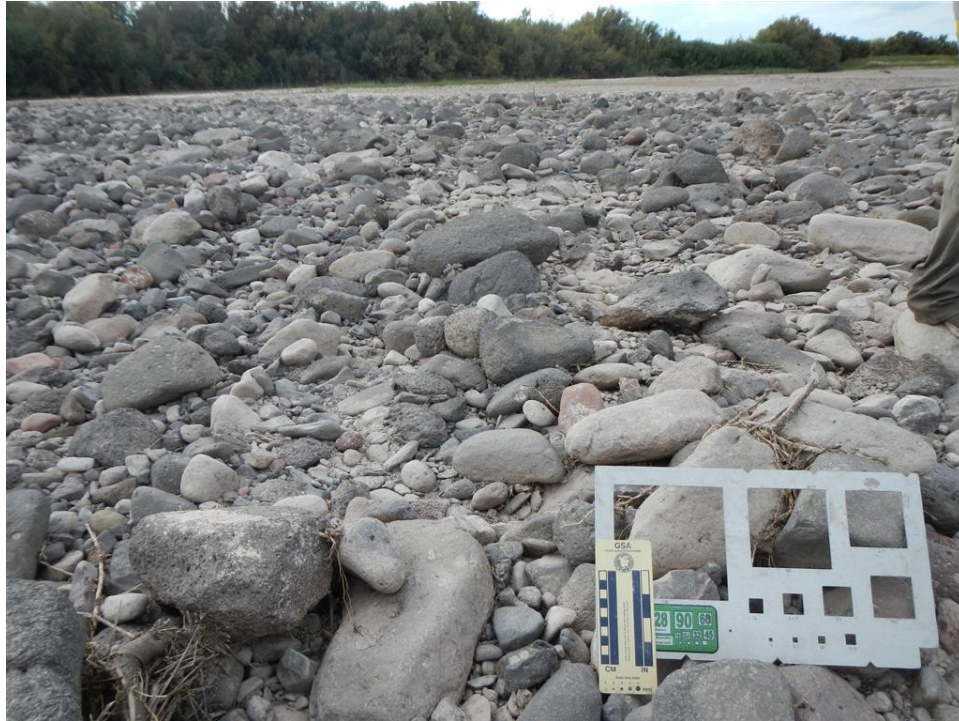
Photo A.41. View of the surface material along the Bignell Arroyo fan that was sampled in Pebble Count PC8.
